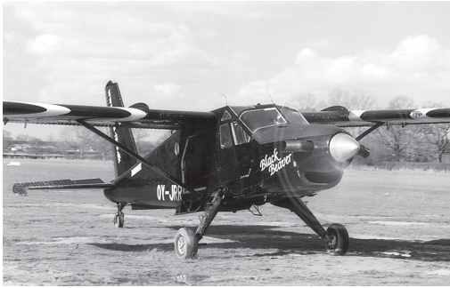
Jim's "other" flying machine. He flies this turbine Beaver for a sky-diving company, Para-Flite. The Beaver carries 10 jumpers and needs only 300m of grass runway to get away
