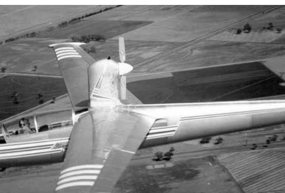
The Motor Blanik modification that was done by Bill Riley at Tocumwal (David did the structural design), flown by Bert Perssons, with wool tufting on the side of the engine cowl to try to locate the source of buffeting on the vertical tail. Bill Riley was flying the camera aircraft and David took the photo. Unfortunately, the added mass of the engine would have halved the fatigue life of the aircraft. However, it was an absolute delight to fly
