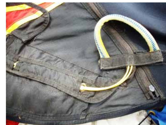
Figure 2: Both cables routed through the RH closing loop – wrong!
