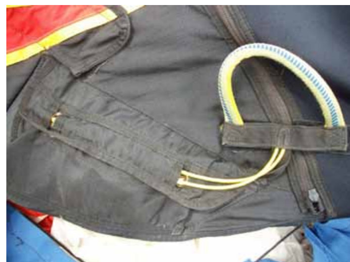
Figure 1: The handle correctly assembled
